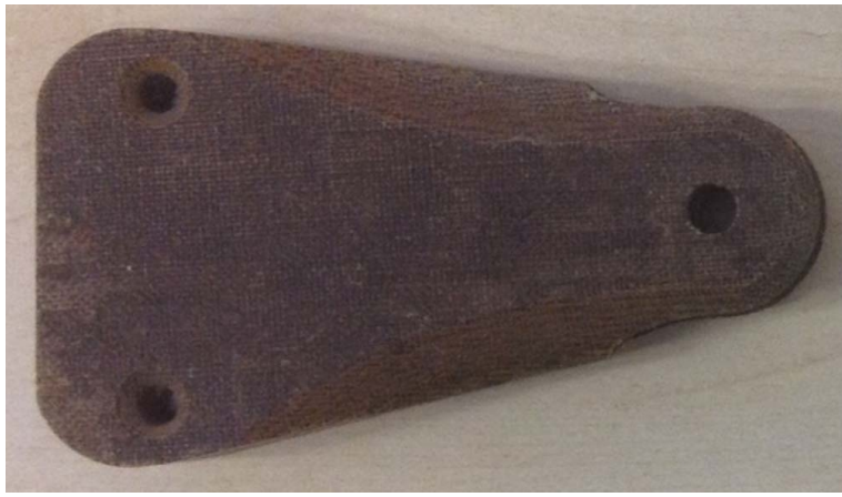
8: The triangular 'pulley insulator' for the HF aerial wire: this had a small guide wheel embedded in the rounded nose [Both images from http://spitfirespares.co.uk/radio.html ]
