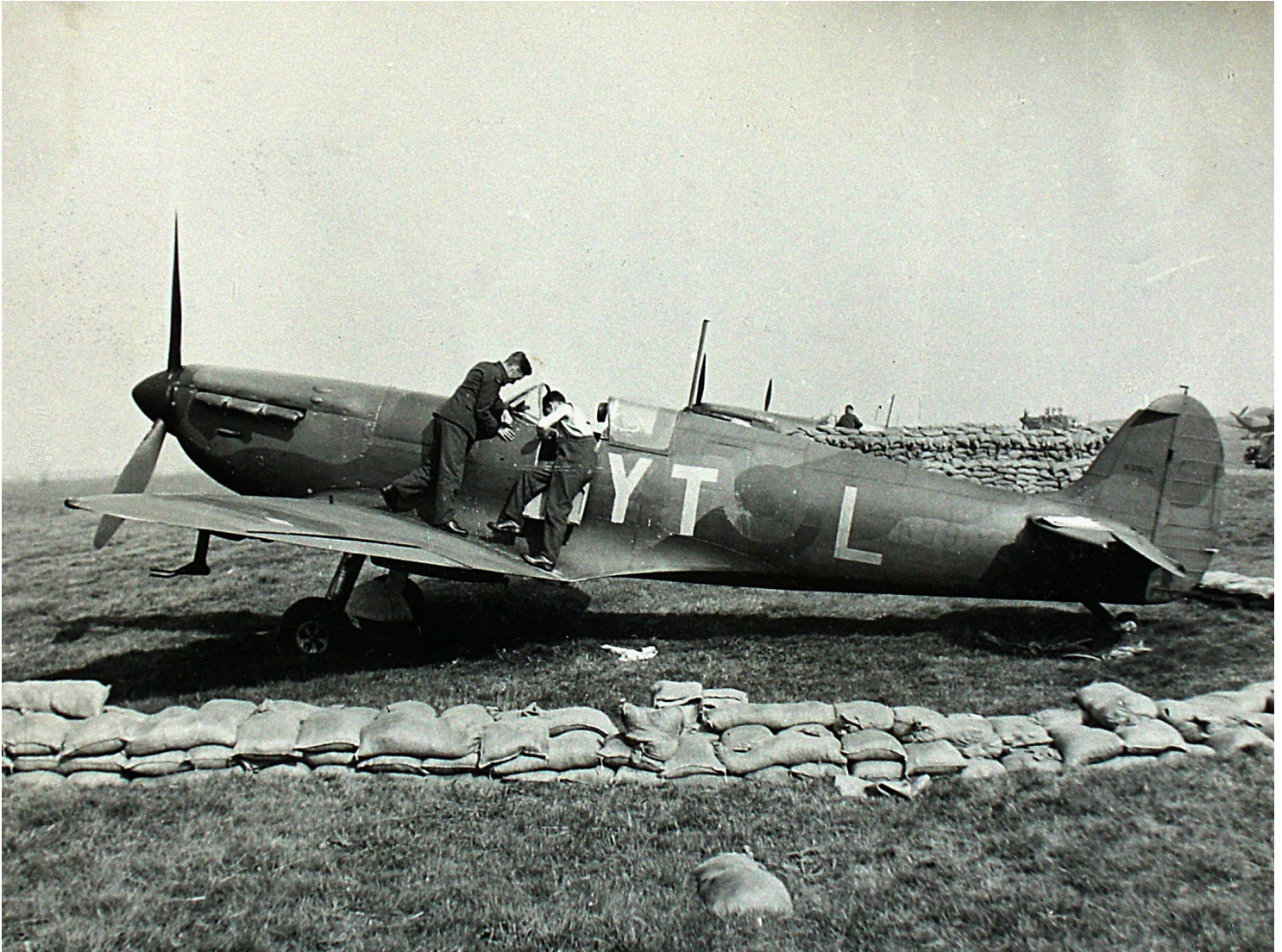
4: An early production Spitfire Mk. I, K9906 of 65 Squadron, with the pole mast and rudder post, with its swivelling insulator. Also note the crudely painted code letters and repainted fuselage roundel. [Photo taken by Sergeant Patrick Hayes. https://www.asisbiz.com/il2/Spitfire/RAF-65Sqn-YT.html https://aviation-safety.net/wikibase/21971 ]
