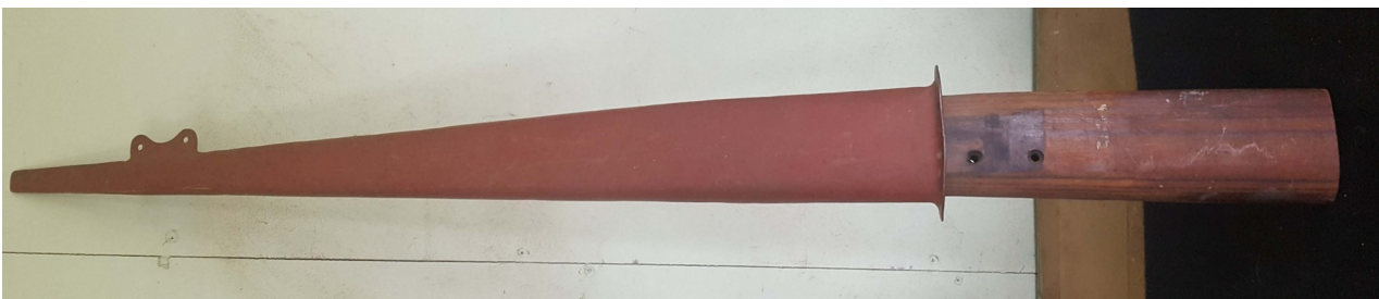
5: The standardised, steel-bodied, wooden-cored mast. The wood core was normally more tapered towards the base to fit in the fuselage anchor point (see 6). Also note the integral, scalloped attachment point for the pulley insulator: it was never deleted, even when the VHF R/Ts were installed. [From: http://spitfirespares.co.uk/radio.html ]
