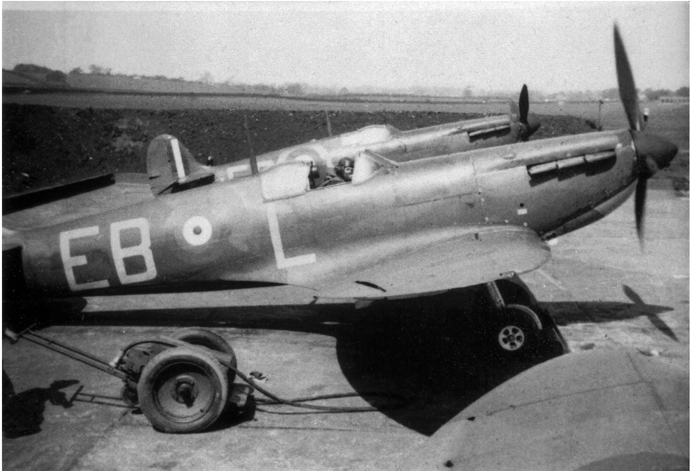
14: Two 41 Squadron Spitfire Is, with the early TR1133 installation, RAF Catterick, late May 1940: EB-L was N3123. The triangular wire guide had been removed from the masts and the rudder post had been deleted on the Spitfire in the background.
