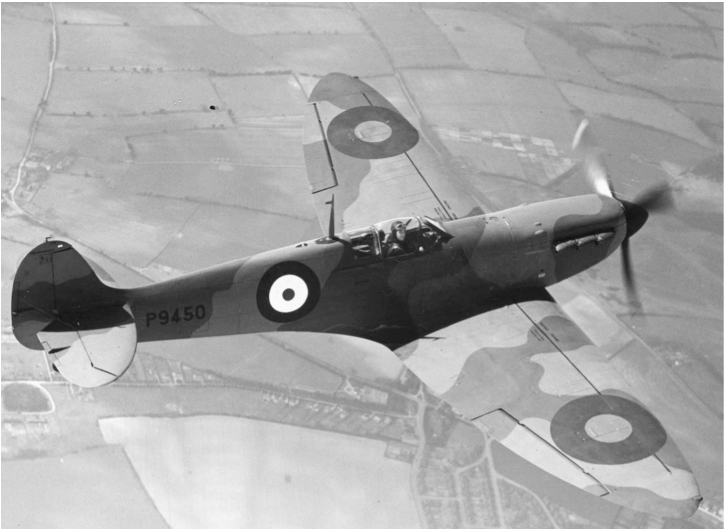
10: P9450 on a factory test flight in April 1940, showing the standardised mast, with the triangular wire guide at the rear and teardrop-shaped base insulator. The insulator was left unpainted and could vary in colour, from black to a dark-brick red. The lead-in for the stainless steel wire can just be seen as a white dot, aft of the mast.
