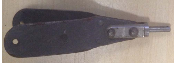
8: The triangular 'pulley insulator' for the HF aerial wire: this had a small guide wheel embedded in the rounded nose [Both images from http://spitfirespares.co.uk/radio.html ]
